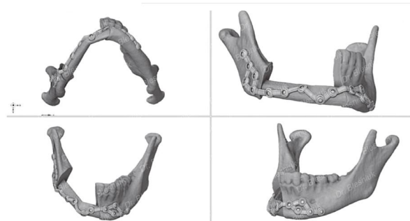
Figure 5 – Stereolithographic models of the lower jaw and pre-modeled individualized titanium osteosynthesis plate, obtained using CAD/CAM technology.
